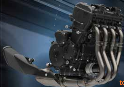
999cm 3 4-stroke, 4-cylinder, liquid-cooled, DOHC engine
